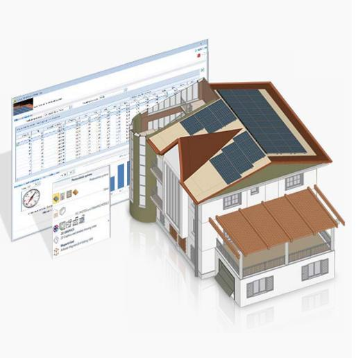
Quickly design and set up your photovoltaic system with a simple to use but powerful 3D BIM modeler Solarius PV offers you the simplest way to design and size PV systems according to your specific needs: 3D/BIM modelling.
